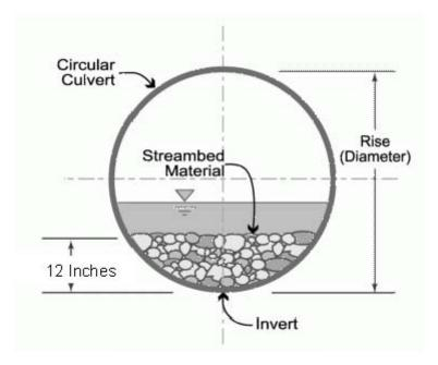
In all other areas: Culverts greater than 48 inches in diameter will be buried at least one foot below the bed of the stream. Culverts 48 inches in diameter or less shall be buried to maintain aquatic passage and to maintain passage during drought or low flow conditions, and every effort shall be made to maintain the existing channel slope.
